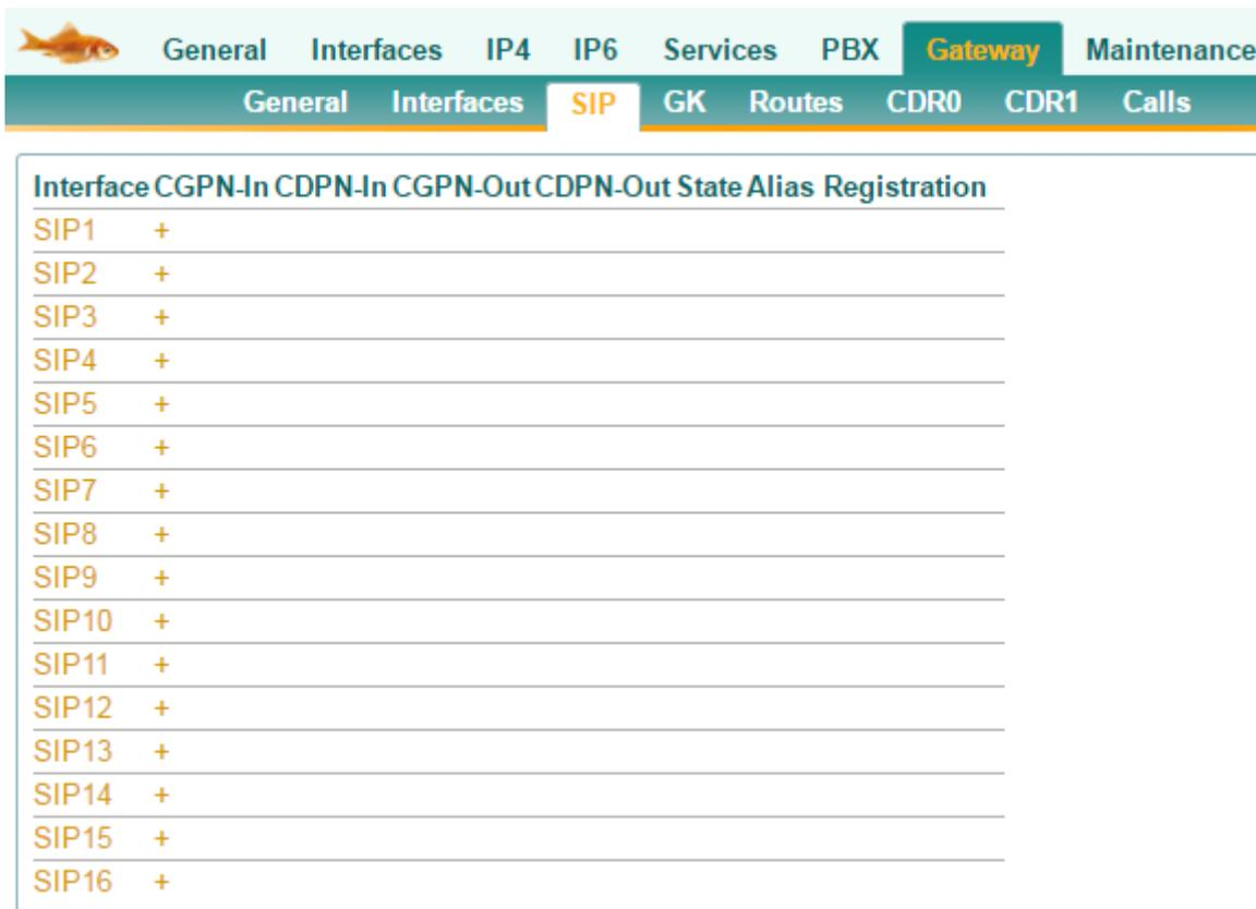
The screenshot shows the configuration interface for a SIP Gateway. The top navigation bar includes 'General', 'Interfaces', 'IP4', 'IP6', 'Services', 'PBX', 'Gateway', and 'Maintenance'. The 'Gateway' tab is selected. Below this, a sub-menu shows 'General', 'Interfaces', 'SIP', 'GK', 'Routes', 'CDR0', 'CDR1', and 'Calls'. The 'SIP' sub-tab is active, displaying a table of SIP interfaces.
